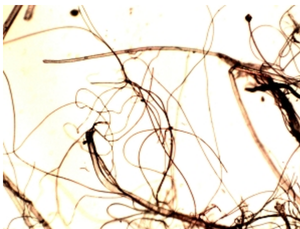
Spider Web Sample – A smoother and more linear structure is observable within the spider webs versus the environmental filament. The differences are not dramatic at this lower level of magnification. Magnification approx. 500x.
